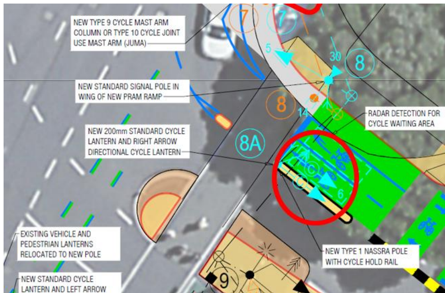
Figure 3-6: Signal group numbers for Bunny Street primary cycle signals missing
