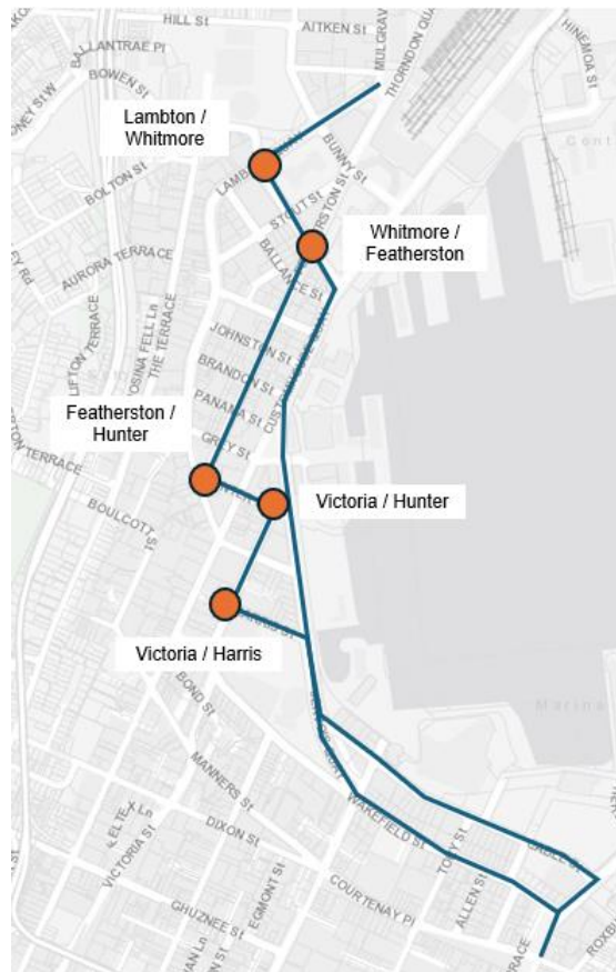
Figure O-1: Intersections where vehicle tracking of an 18m articulated vehicle has been undertaken (blue line represents the preferred interim option bus route)
