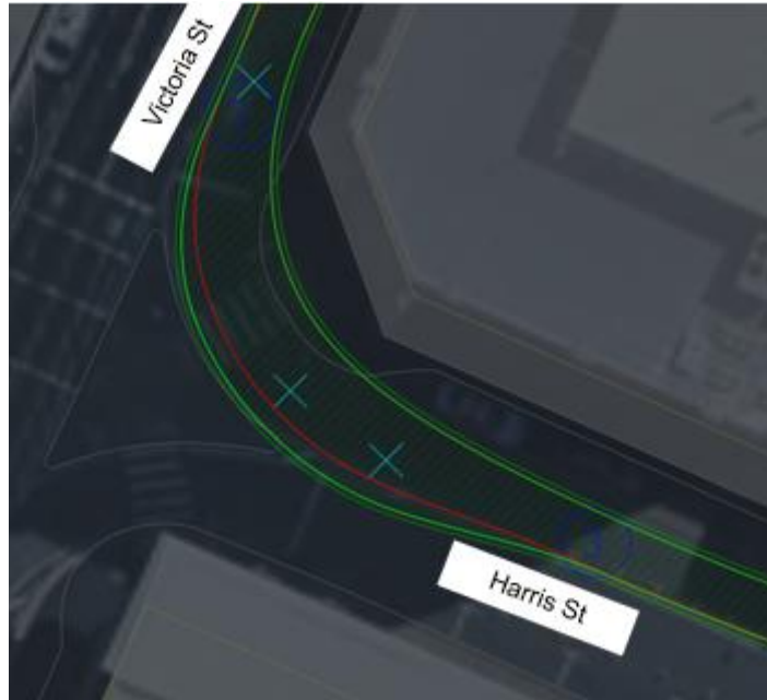
Figure O-6: Vehicle tracking for vehicles turning left from Victoria Street to Harris Street
