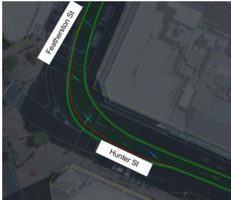
Figure O-4: Vehicle tracking for a vehicle turning right from Featherston Street to Hunter Street
