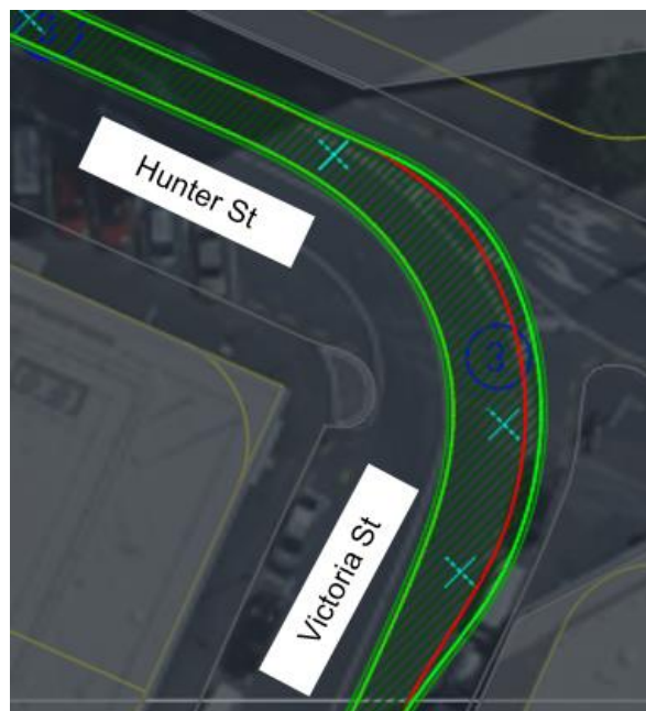
Figure O-5: Vehicle tracking in both directions between Victoria Street and Hunter Street
