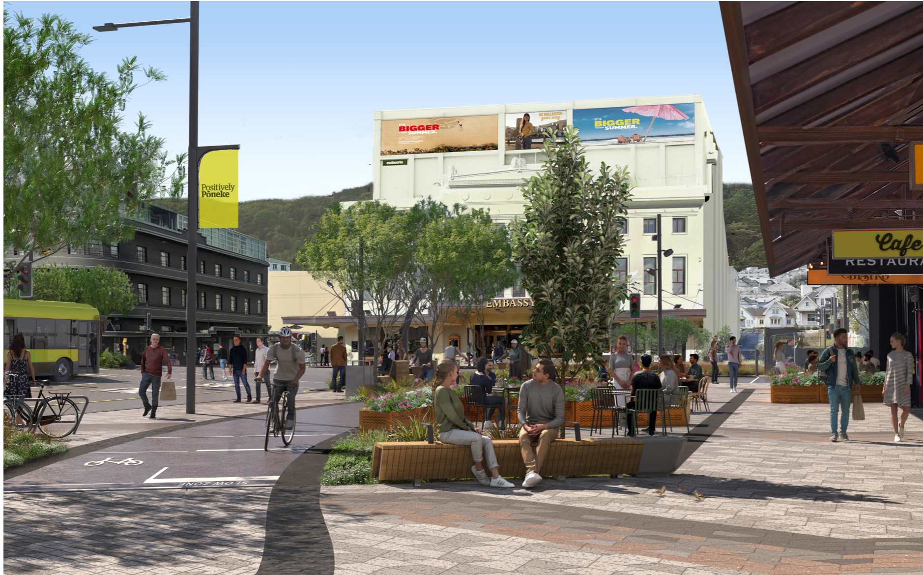
View H - View of the Southside of Courtenay Place from Cambridge Terrace showing the dedicated 4.0m wide footpath and the eating areas beyond.
