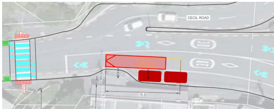
Figure 14: #100 Bus stop outside adjacent kerbside parking.
